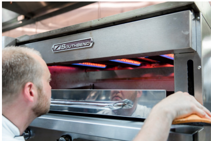
Chef Will Morris manipulates the handle on this typical restaurant broiler. He can raise or lower the rack without having to touch it.
