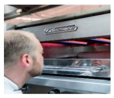
Deck ovens use conduction heat, a process in which heat travels directly from a hot stone or deck to the food. Deck ovens also utilize radiant heat, a process that incorporates infrared heat waves to penetrate food, heating it throughout.
