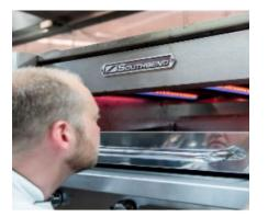
Deck ovens use conduction heat, a process in which heat travels directly from a hot stone or deck to the food. Deck ovens also utilize radiant heat, a process that incorporates infrared heat waves to penetrate food, heating it throughout.
